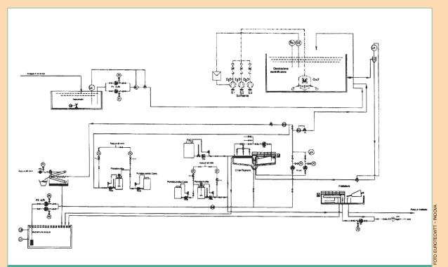
Aerobic plant flow chart for the treatment of regeneration eluates from fruit juices demineralization plant
