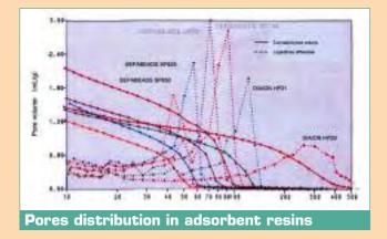
stances. The pores dimensions and surface area are graded according to the type of adsorbent resins. There are several applications in food industry oriented to removal of undesired organic substances and to recovery of valuable organic substances. These are products in constant development, therefore the new and unknown applications are many. Adsorbent resins reversibly adsorb polar organic molecules as polyhydric phenols, organic
