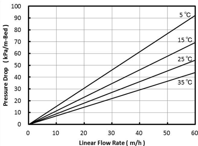
Fig. 1 Pressure Drop of CRBT03
