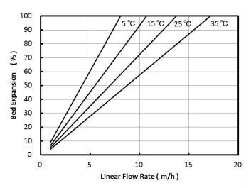
Fig. 2 Bed Expansion of RCP160M
