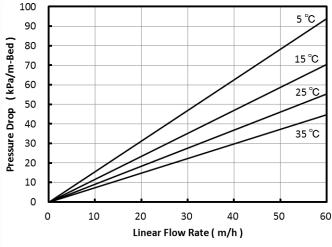
Fig. 1 Pressure Drop of RCP160M
