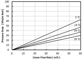
Fig. 1 Pressure Drop of SANUPB
