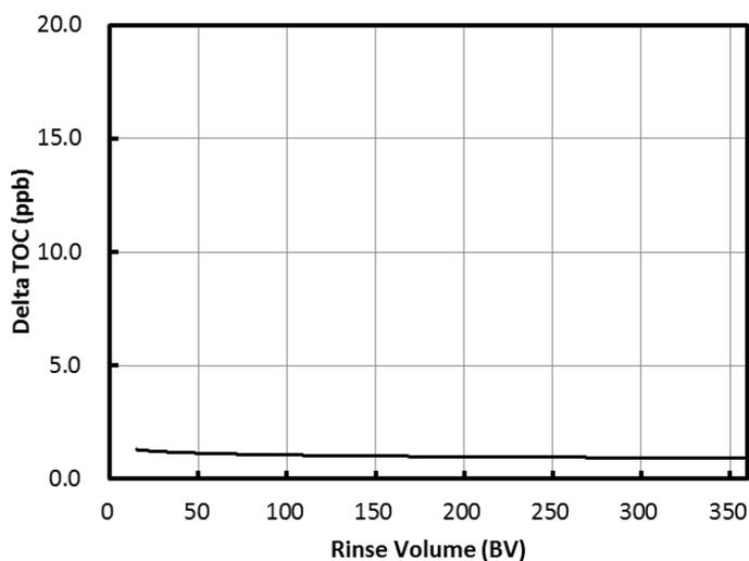
**Fig. 4 Delta TOC versus Rinse Volume for SAT20L**
