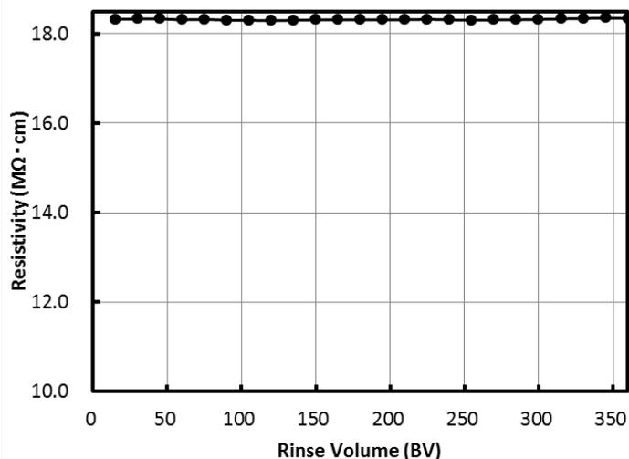
**Fig. 3 Resistivity versus Rinse Volume for SAT20L**
