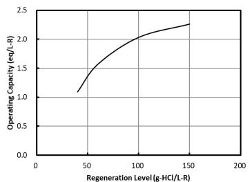
Fig. 3 Operational Capacity Data of SK110
