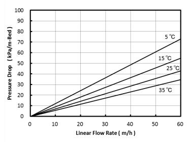
Fig. 1 Pressure Drop of SK110
