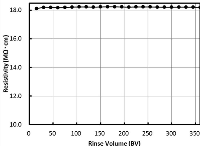
**Fig. 2 Resistivity versus Rinse Volume for SMNUPB**
