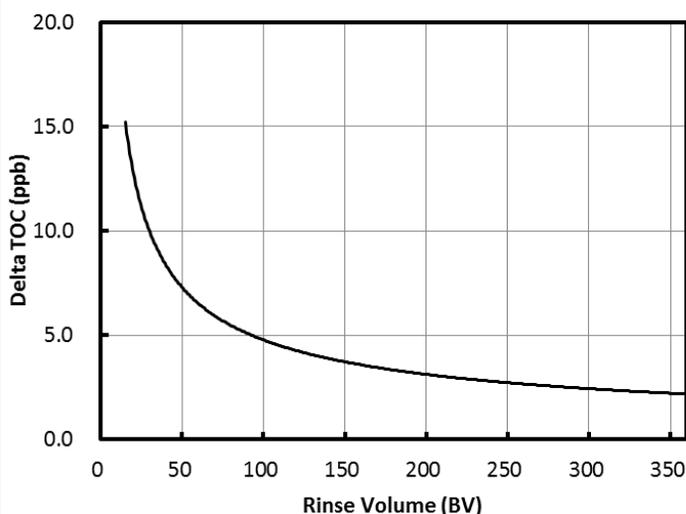
**Fig. 3 Delta TOC versus Rinse Volume for SMNUPB**
