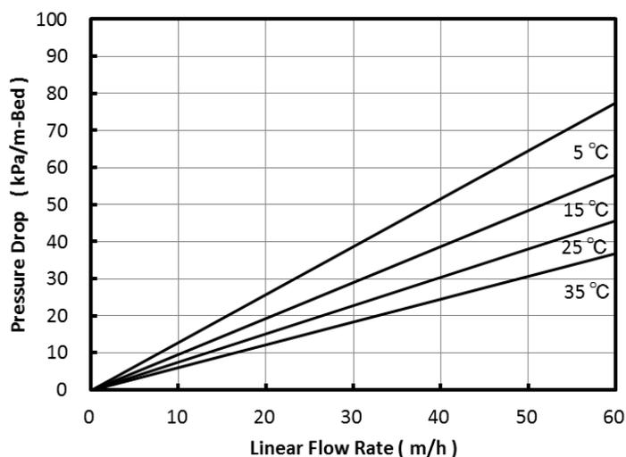
Fig. 1 Pressure Drop of UBA100OHP
