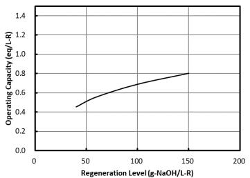
Fig. 3 Operational Capacity Data of UBA120 Regenerant: 4 % NaOH
