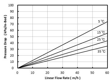
Fig. 1 Pressure Drop of UBA120
