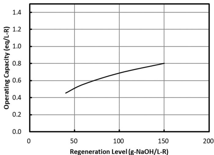
**Fig. 3 Operational Capacity Data of UBA120A**
