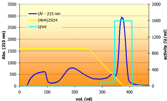
**Blue line:** elution profile; **Yellow line:** buffer elution gradient;
