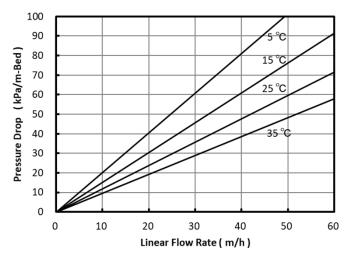
Fig. 2 Pressure Drop of SP850
