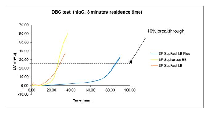
**Figure 2**: Dynamic binding capacity (DBC) test was conducted by loading human polyclonal immunoglobulin (i.e. hIgG, molecular weight ca 150,000 dalton) until it reached over 10% breakthrough. Each resin was packed to a 11mm i.d. column to final bed volume of 2 ml. The running flowrate was controlled to give a residence time of 3 minutes. Buffer: 50 mM sodium acetate, pH 4.7. Protein solution: 1 mg/ml
