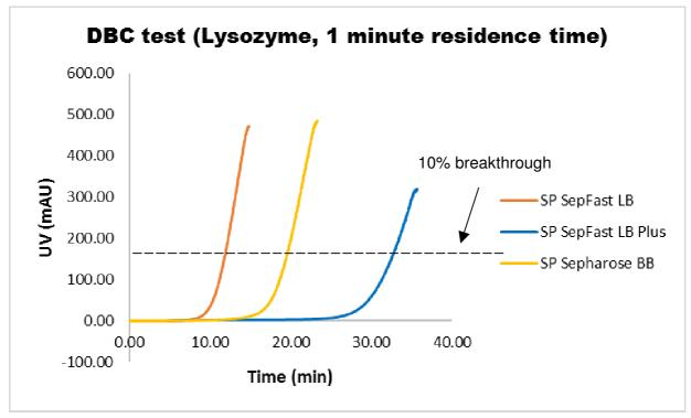
**Figure 3**: Dynamic binding capacity (DBC) test was conducted by loading lysozyme (molecular weight ca 14,000 dalton) until it reached over 10% breakthrough. Each resin was packed to a 11mm i.d. column to final bed volume of 2 ml. The running flowrate was controlled to give a residence time of 3 minutes (0.7 ml/min) or 1 minute (2 ml/min). Buffer: 50 mM sodium phosphate, pH 7.2. Protein solution: 5 mg/ml.
