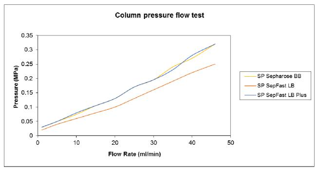
**Figure 1:** The pressure flow property was tested by packing each resin to a 11mm i.d. column to final 2 ml bed. The liquid phase is deionised water and the test was done at room temperature.
