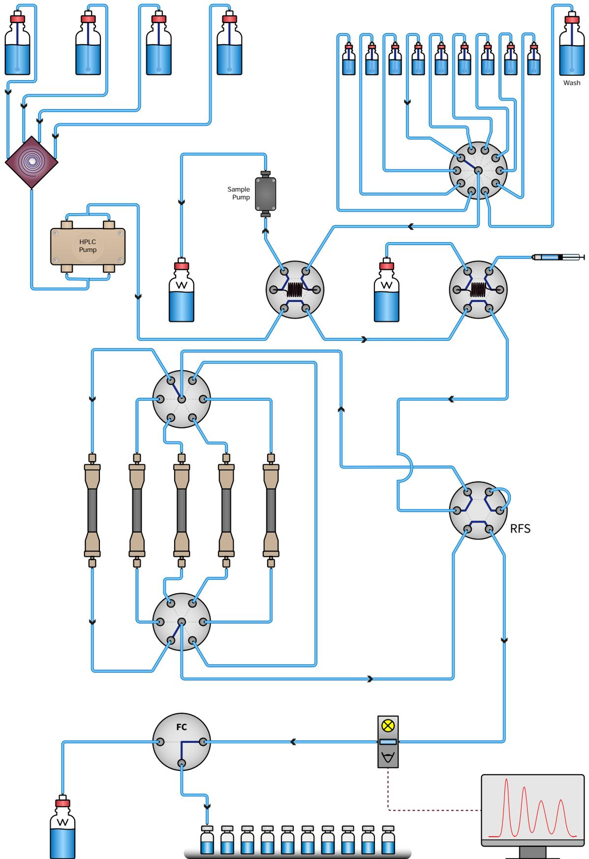
*A low pressure quaternary gradient system with manual and automatic injection. Column switching up to 6 columns, or 5 columns and one bypass for flushing or sanitizing routines. Reversed flow switching (RFS) for counter-current elution or column regeneration. Fraction collector.*
