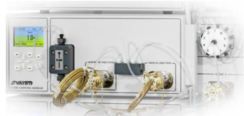
The S 5400 Sampling Module with built-in sampling pump and two separate injection valves offers manual syringe injection and variable volume injection controlled by the sampling pump.
