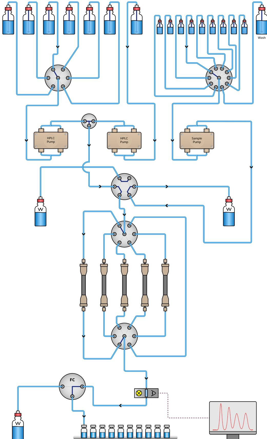
A **binary high pressure gradient system** with additional 6-channel buffer/eluent selection for the primary pump. A sampling pump for large volume sample injection and a sampling valve for connecting up to 10 sample containers. Column switching up to 6 columns, or 5 columns and one bypass for flushing or sanitizing routines. Fraction collector.
