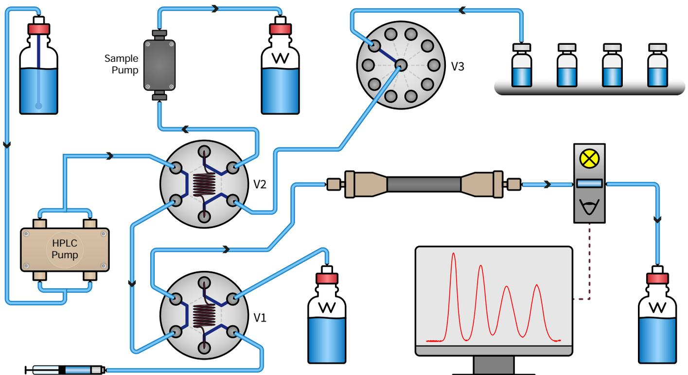
Shown above: the S 5400 sampling flow path. Valve 1 is the manual injection valve. Valve 2 is the automatic injection valve. Valve 1, valve 2 and the sample pump are integral parts of the S 5400 sampling module. Valve 3 is the optional external valve for automatic sampling of up to 10 samples. The sample inlet lines to the 10-port valve can be connected to any external sample container or to the optional S 5405 sample loading rack with 10 closed tubes of 50 ml.
