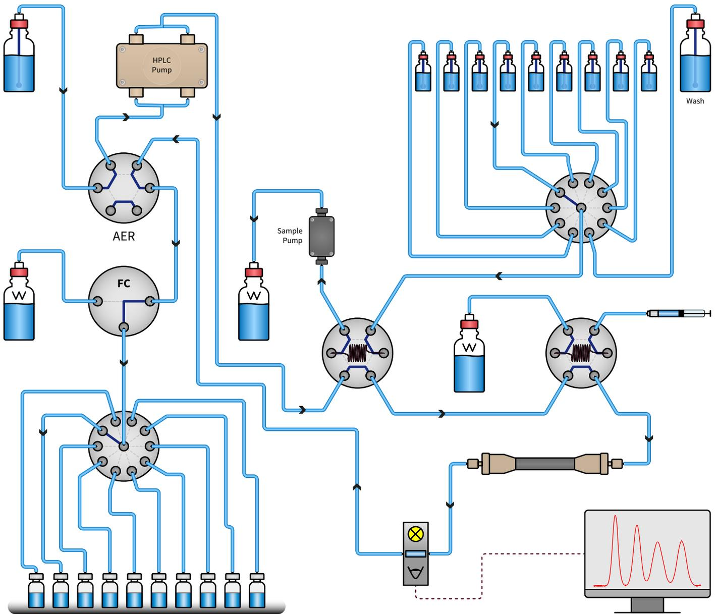
An **isocratic system** with automatic eluent recycling (AER) possibility and manual and automatic sample injection. Fraction collection with a 10 port valve enabling large volume collection, useful for stacked (repeating) sample injection routines.
